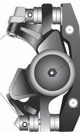
Adjustment screw for limiting play between brake disc and brake pad
