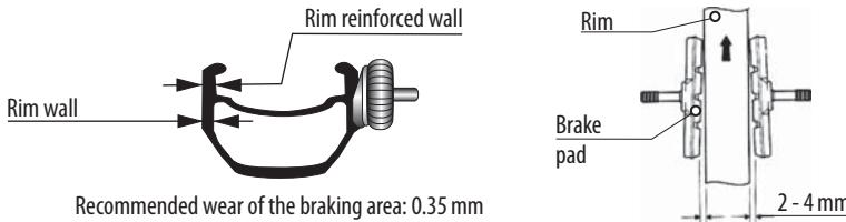
Keep the brake pads adjusted in a distance of 2-4 mm from the rim with a slight gradient as indicated in the figure. Check their wear and replace them if necessary. Clean oil or dirt accumulated on the rim and brake shoes.
