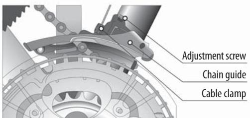
chainring to a larger one by moving the left-hand shifter forward. You will learn soon what positions should be used for different riding conditions. You will learn it through training only. Do not try to change gears while applying heavy pressure on the pedals. Never pedal backward when changing gears. This could result in the chain slipping down.
