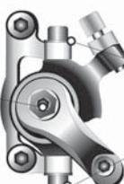
Adjustment of tilt of brake yoke with respect to brake disc
